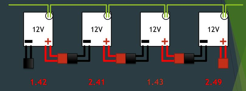
In the example above, a possible safety or hazard condition exists that can occur during recharging. A Lithionics Battery 'Rescue Charger' is needed to gently begin charging the batteries at a special low voltage using a special algorithm. Purchase a Rescue Charger from Lithionics Battery only.
