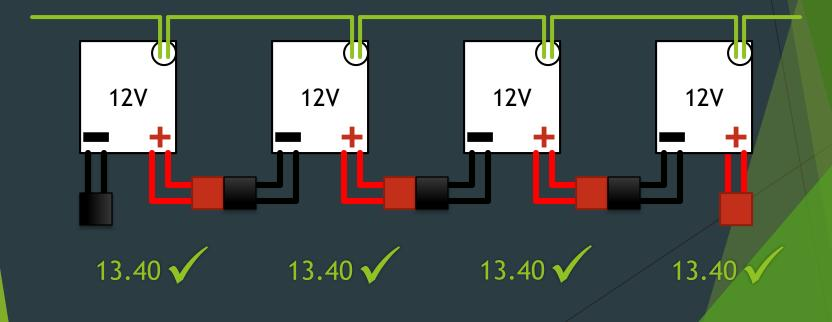
If you now have module-to-module compatible voltages and voltage-balance, and, you have continuity, HOWEVER, the master NeverDie® BMS will not power-up, contact Lithionics Battery for support on how to field-diagnose the master BMS.
