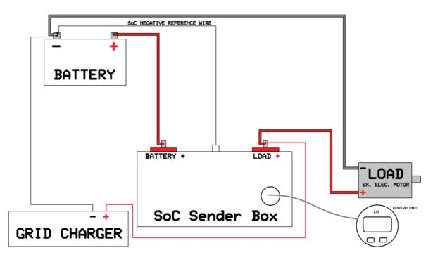
ALL CHARGE & DISCHARGE LOADS MUST BE CONNECTED TO LOAD +
