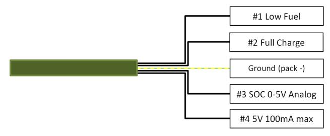
**#1 Low Fuel** - The Low Fuel output circuit is 0V when inactive and 5V when active. It corresponds to the Low Fuel setting in the user menu.
