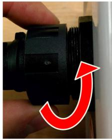
4. Now turn the ring <u>clock-wise</u> to begin screwing the ring down. Keep note of any excess friction which may indicate it is being cross-threaded. If this occurs stop immediately, unscrew the ring and start over. Inspect the ring to be "square" compared to the panel.
