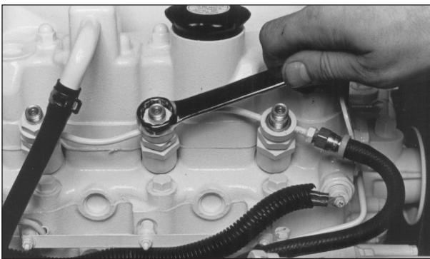
Figure 9: Remove return line nuts.
