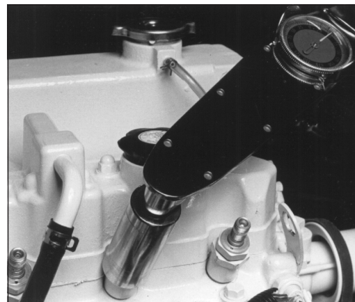
Figure 13: Reinstall injector. Torque to proper tightness.
