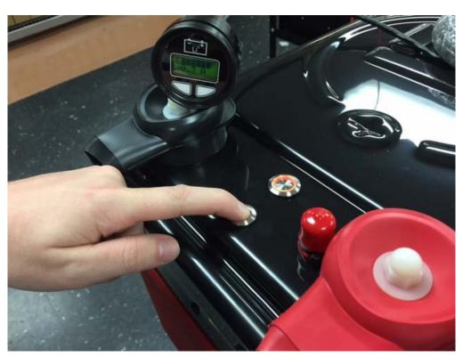
Storage MODE: Power-Down the SOC Gage and the Battery for Long Term Storage: Press-Release the MAIN POWER Switch (to UP Position)
