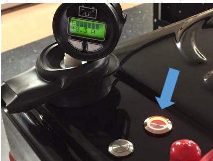
Step 3: Press the RESET Button for 1 Second and Notice the Contactor Latches. The Battery is Now in the LIVE or ON State
