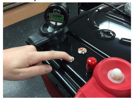
Power Cycle OFF, Leaves SOC "ON": Press the Reset Button for <u>5 Full Seconds</u> Then Release. Battery is SAFE for Terminal Voltage
