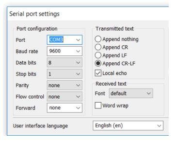
Any terminal emulator software with COM port support can be used to communicate with BMS. We recommend free software called Termite, which allows data logging and has bidirectional command interface:
