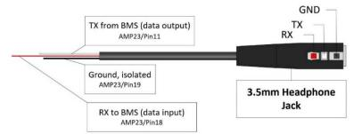
NOTE: If your BMS is equipped with a Bluetooth module, then external Serial Port is disabled. Since Bluetooth operates over serial port internally, only one option can be enabled, either wired Serial Port or wireless Bluetooth module. Specific configuration is assigned during BMS manufacturing and cannot be changed by a customer. Please contact Lithionics Battery or your dealer for details.
