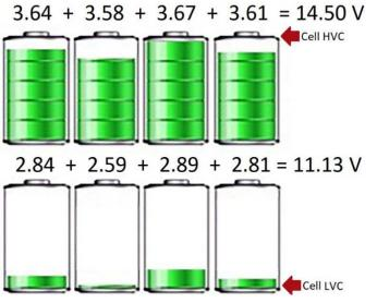
Picture on the left illustrates the cell level and the pack level voltages. Due to manufacturing tolerances and environmental factors individual cell voltages may not always be the same, so the BMS must employ both cell level (MiniBMS<sup>®</sup>) and pack level (NeverDie<sup>®</sup> BMS) triggers for protection events such as HVC and LVC. Our BMS also works to minimize those voltage differences in a process called "balancing", which occurs at the end of each full charge cycle.
