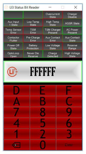
Lithionics Battery has developed the **Li3 Status Bit Reader** application for Windows and Android platforms, which makes it easy to visualize status of each bit by typing in the System Status value and observing color coded table of bit values, see example below. You can download these applications from http://www.lithionicsbattery.com/user-guides/
