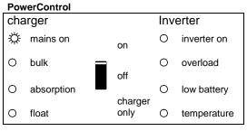
The AC input is switched through. The AC output current is equal to the preset maximum input current. The charge current is reduced to 0.
