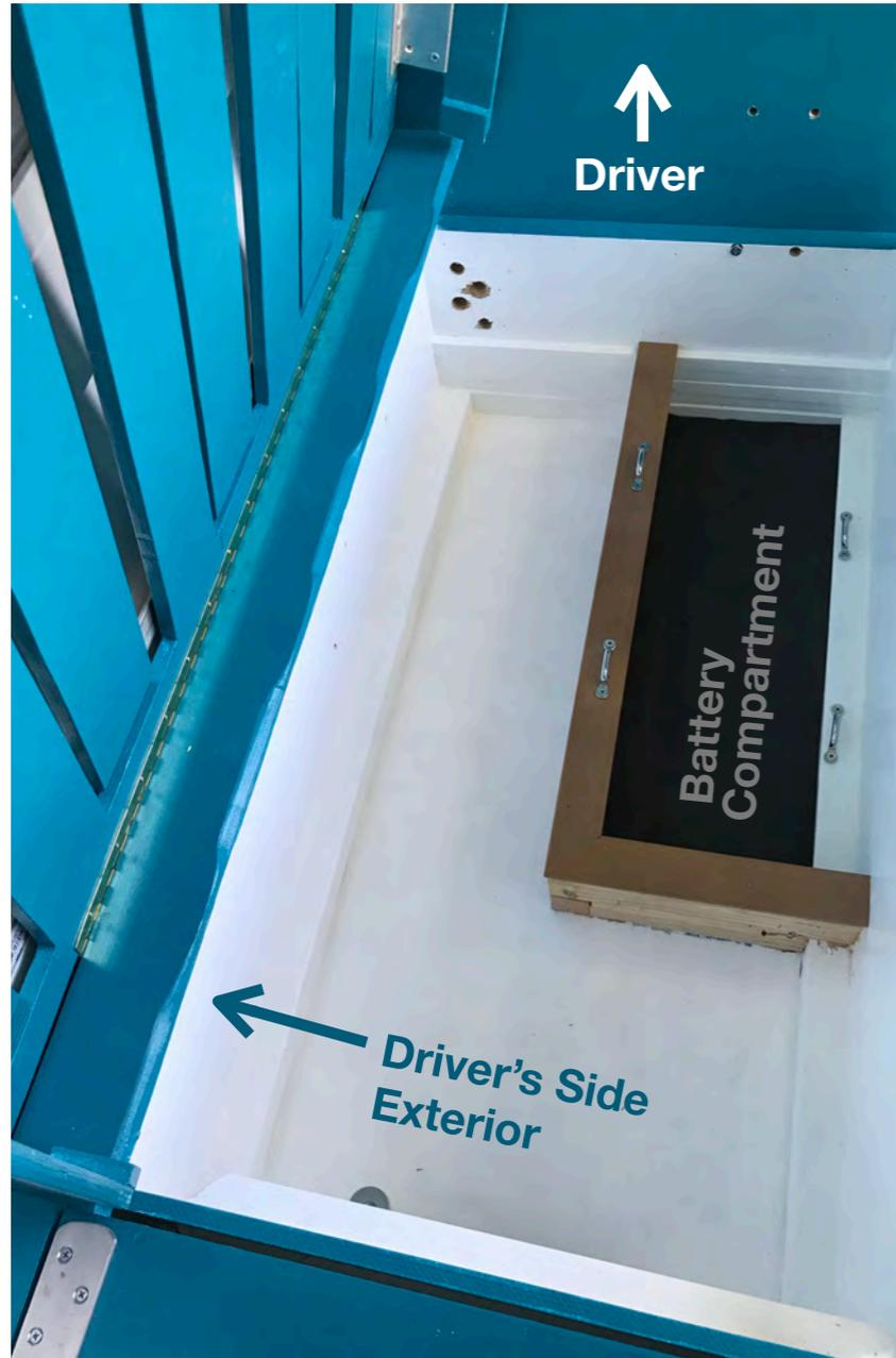
Battery compartment with 20psi foam mat and battery securing straps. Located below sofa-bed, behind driver, & away from van exterior (safeguarding against collision-related damage).
