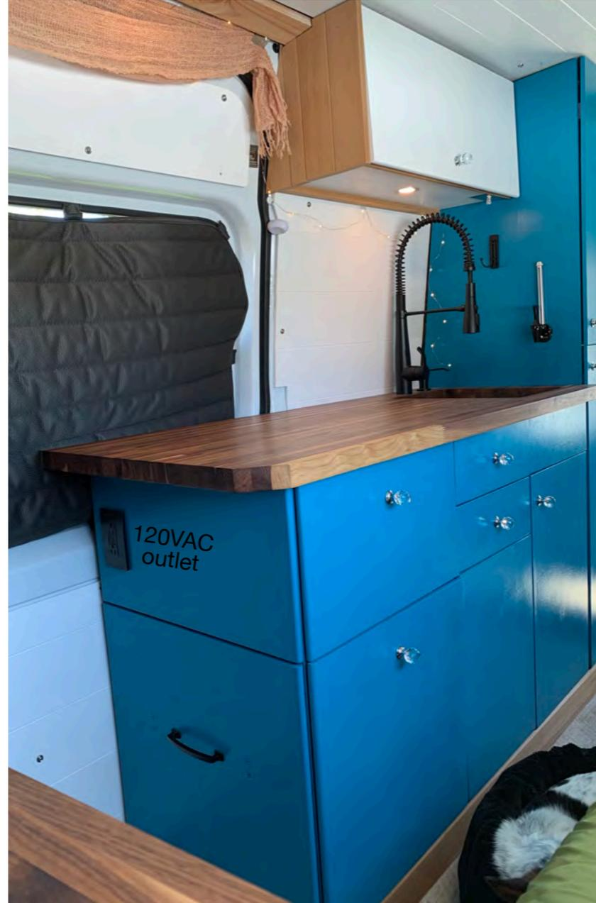
Kitchen cabinet, adjacent to sliding door. Cabinet houses: refrigerator, water pump, and 120VAC receptacle for inductive cooktop.
