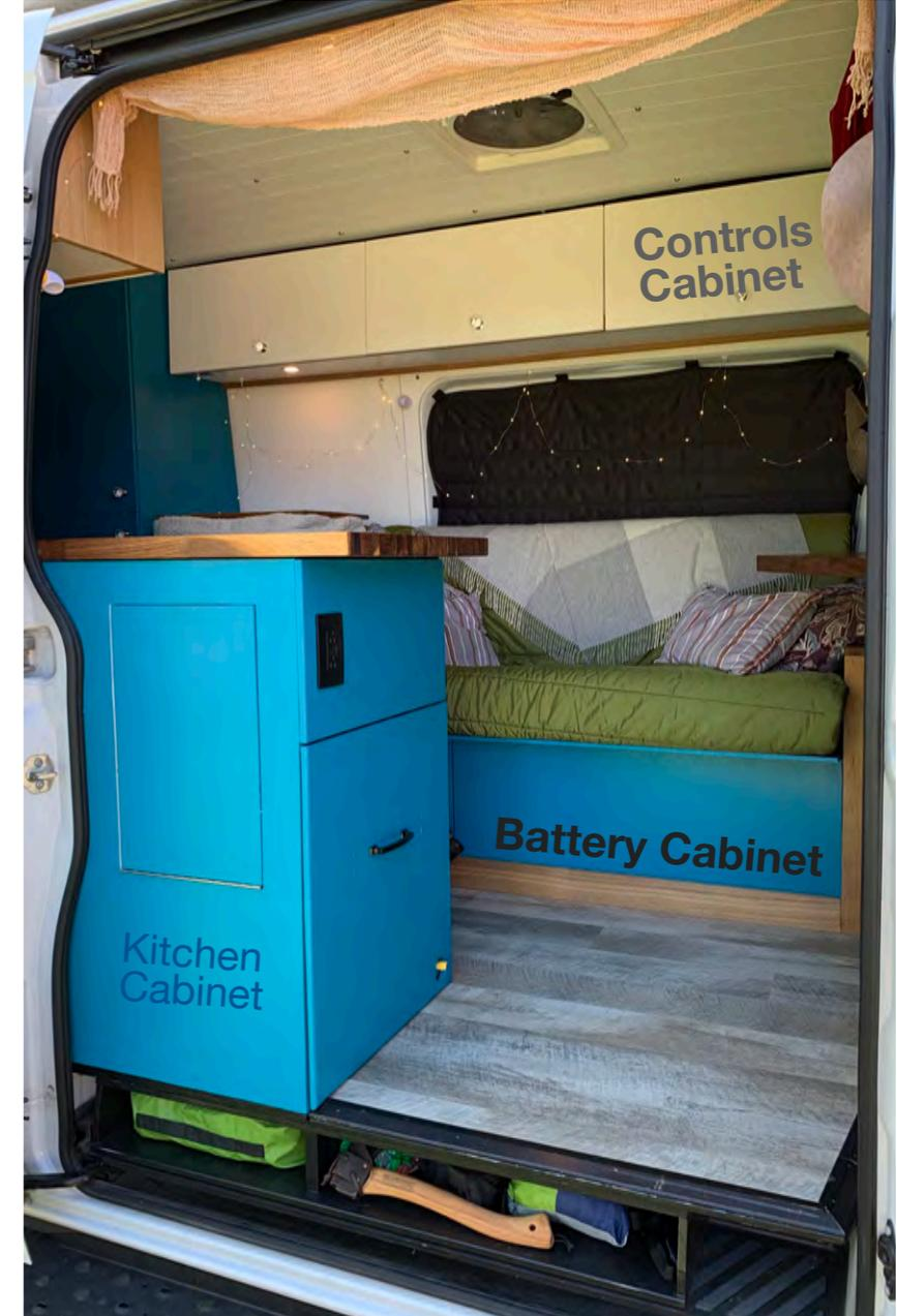
View from sliding door, past kitchen cabinet, to sofa-bed; which houses battery, solar controller, inverter and all associated fuses / busbars. Overhead cabinet contains fuse + breaker box.
