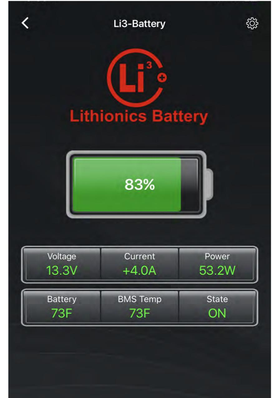
User interface of the "Li3 Battery" app. Enables user to monitor system parameters. In the above case, battery is in bulk charge and sky is overcast (low power input of 53.2W).
