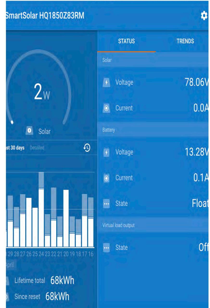
UI of the "VictronConnect" app, which allows user to program the solar controller and to monitor system parameters. In the above case, battery is in float.
