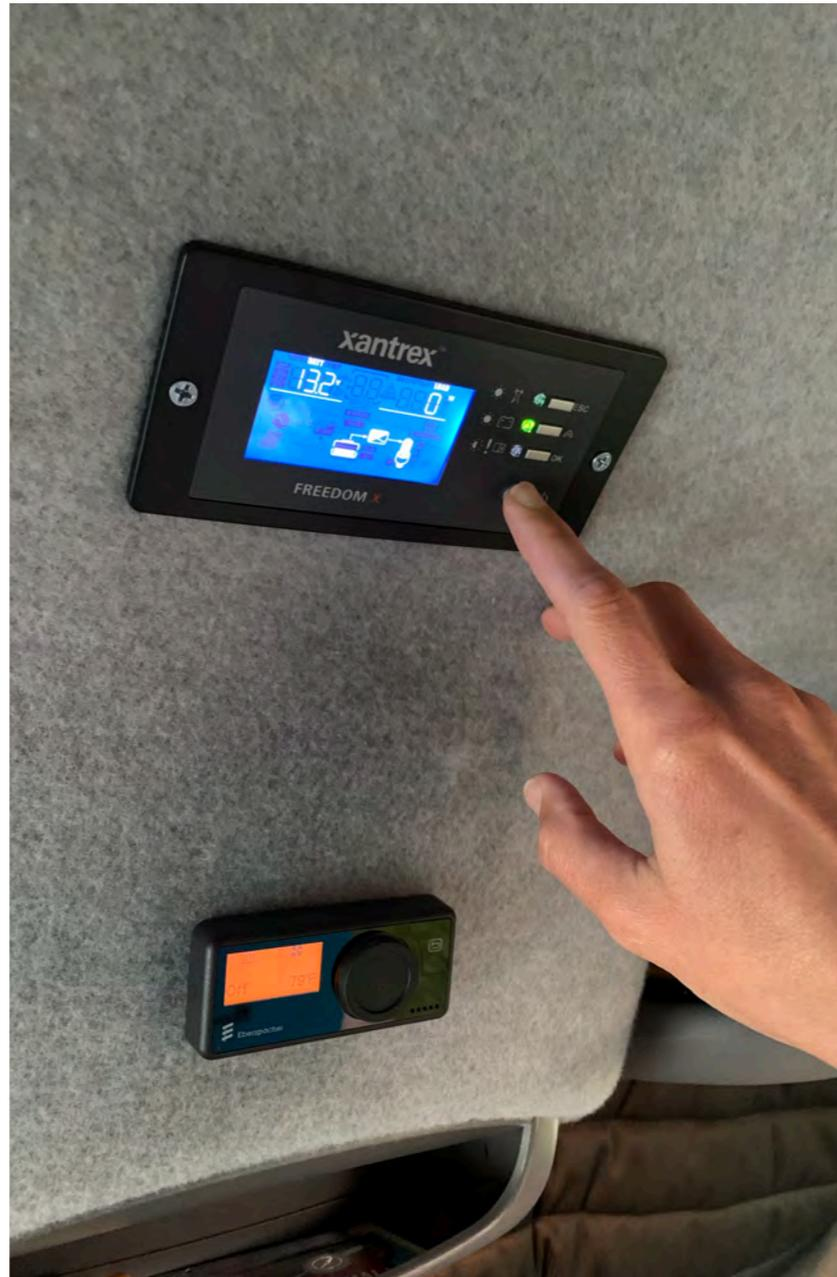
Remote panel for Xantrex Freedom XC 2000 installed overhead, in cab headliner. Inverters are best kept "OFF" when not in use. Thus, a highly visible location (such as this) is ideal.
