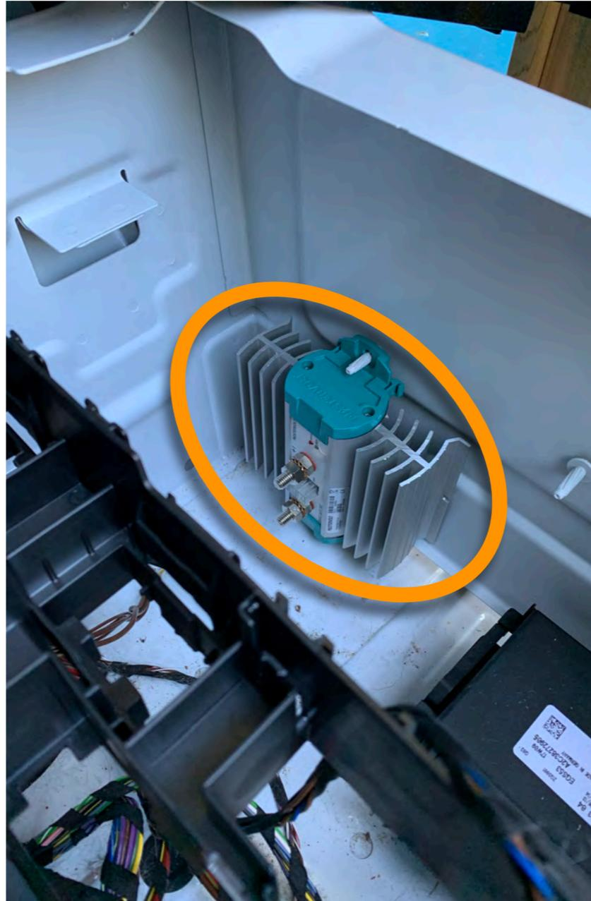
Close-up view of final mounting for Charge Mate Pro40 in seat pedestal. Note: this unit limits current to 40amps, per Mercedes recommendations.
